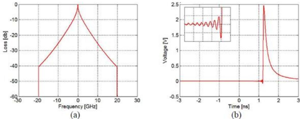
Figure 1: (a) Bandwidth limited insertion loss of PCB Trace (b) Corresponding impulse response with ringing.
