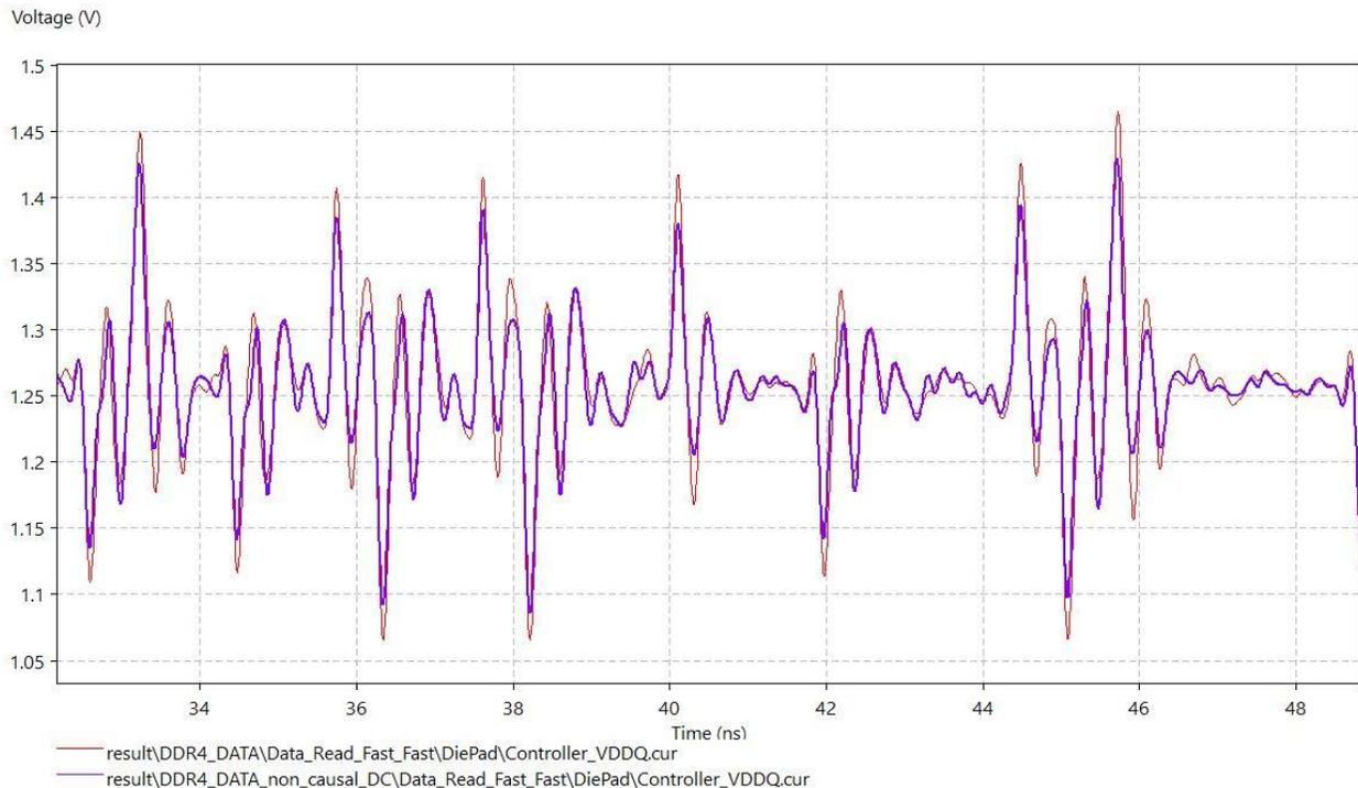
**Figure 5: IO Supply ripple comparison for Causal & non-Causal PDNs during Reads.**
