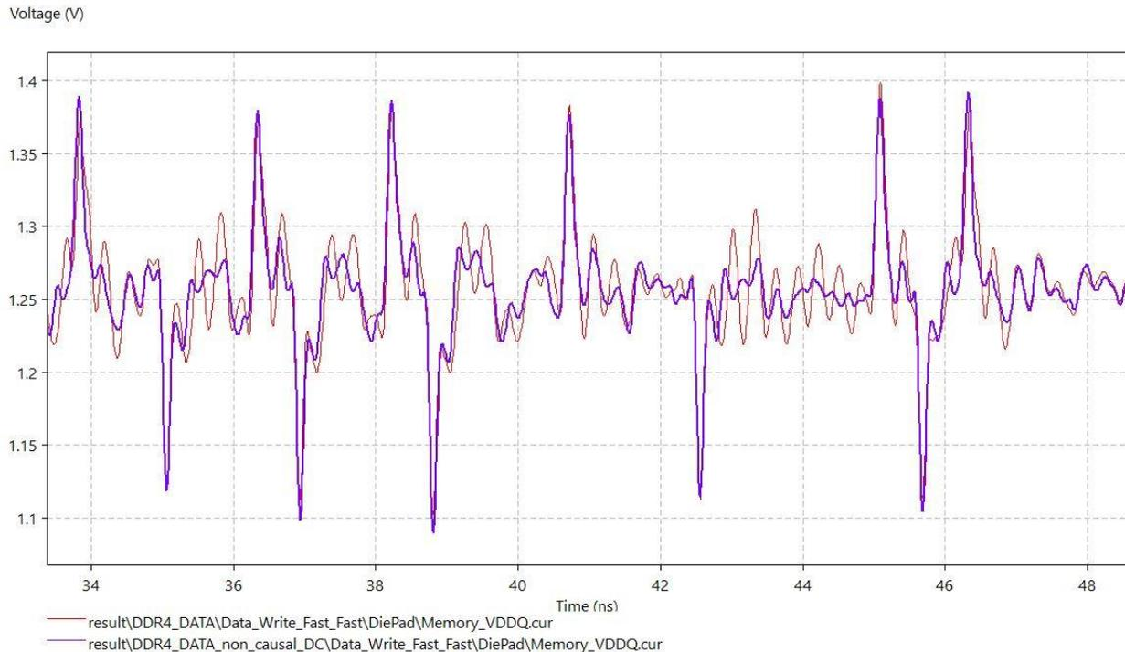
*Figure 6: IO Supply ripple comparison for Causal & non-Causal PDNs during Writes.*
