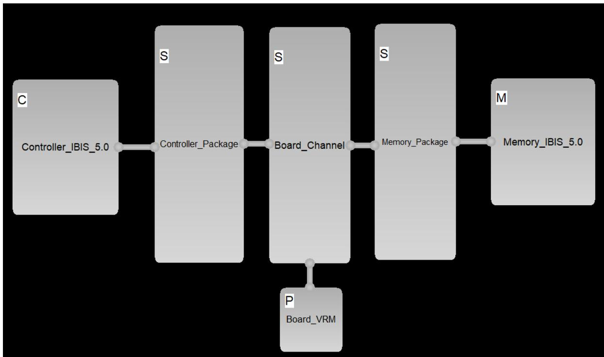
Figure 4: Cascading Causal Channel Models.
