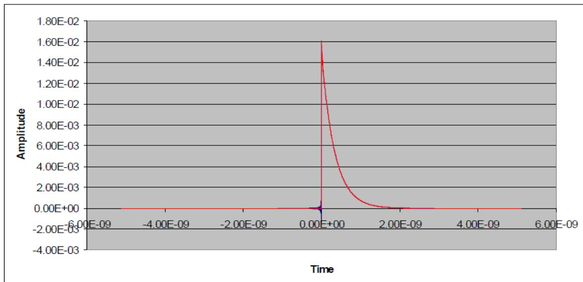
Figure 3: Time domain response with and without non-causal part.
