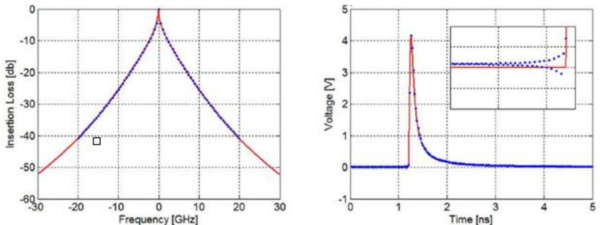
Figure 2: IFT & DIFT of Continuous & Sampled Bandwidth limited S-parameters.
