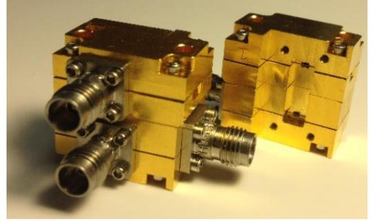
Fig. 6: Complete assembly of DC-35-67GHz hybrid diplexer
