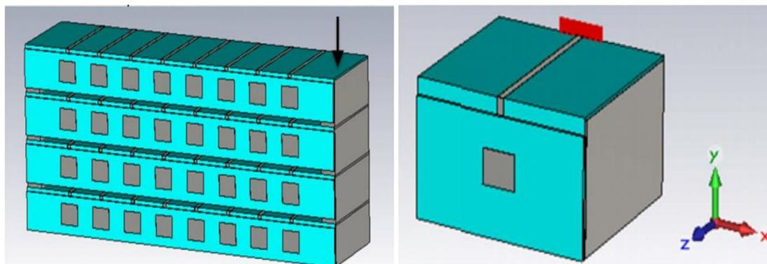
Figure 6 - Eight element array of stacked patch antenna (left), Single element of patch antenna with folded LCP substrate (right)
