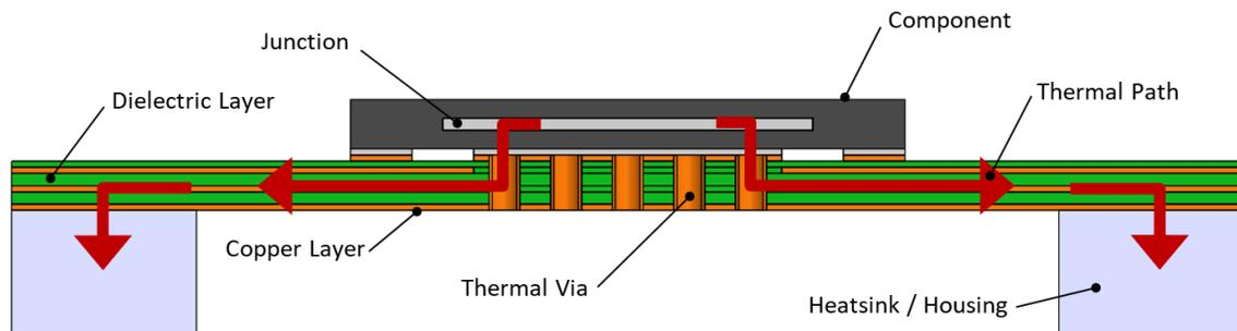
Figure 3 - Standard Thermal Dissipation Case
