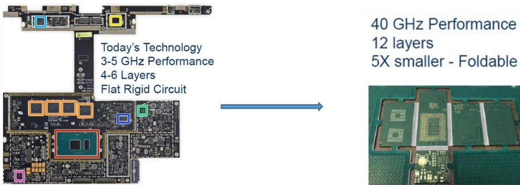
Figure 1 – Miniaturization of a Printed Circuit Board using LCP
