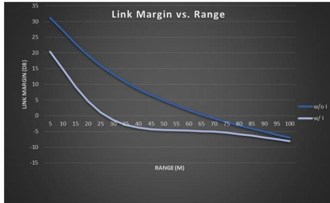
Fig. 8. Vehicle to street Infrastructure link budget analysis results using ANSYS EMIT [9] at 5.9GHz.
