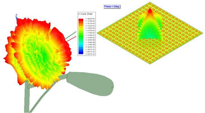
Fig. 6. Conventional patch antenna array in free space (right) and on electrically large platform like light pole (left).
