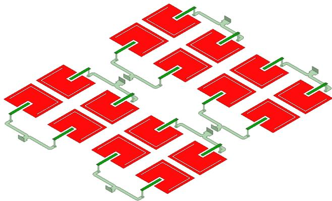
Fig. 5. Early design stage of a section of NxN capacitive coupled microstrip fed patch antenna where microstrip feeding network is printed on the bottom face of two-layer back to back substrates.
