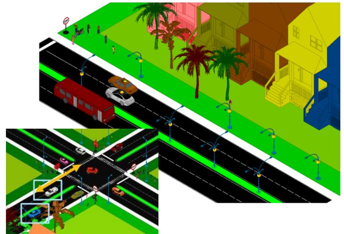
Fig. 7. Modeled street intersection for V2X communications with 5G array implementations.
