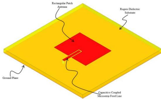
Fig. 1. Complete model of single element capacitive gap coupled microstrip feed patch antenna.
