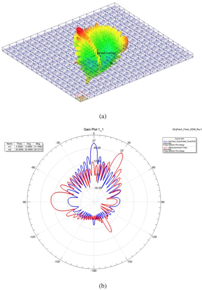
Fig. 4. (a) Conventional Finite Rectangular Patch Antenna Array operating at 28GHz design using ANSYS HFSS Domain Decomposition Methodology, (b) Antenna Array Beam steering using ANSYS HFSS tool kit.
