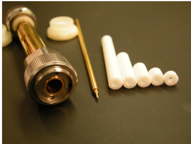
Figure #3: Photo of MMC 2653D 7mm airline and PTFE beads
