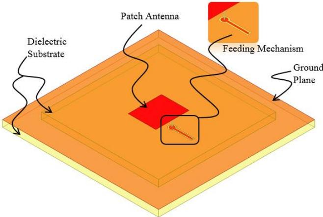
Fig. 1. Proposed Probe-CPW Fed Patch Antenna simulated geometry.
