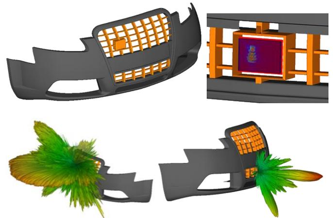
Fig. 4. Implemented radar array installation on front car bumper. Far field TX/RX subarray patterns installed performance.
