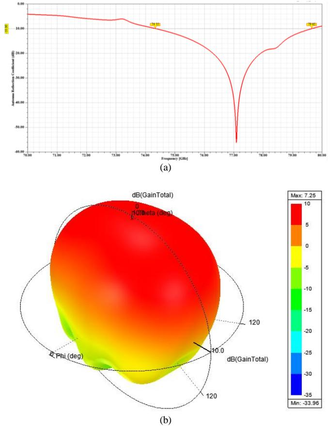
Fig. 2. (a) Proposed patch antenna reflection coefficient, (b) far field 3D polar gain plot.
