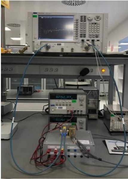
Fig. 2. YIG filter measurement setup.
