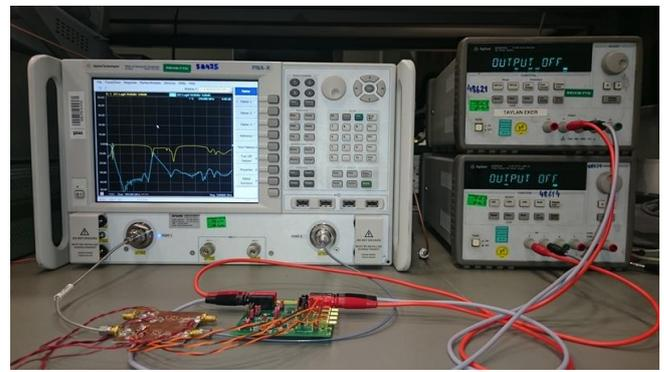
Fig.4 Tunable Filter Measurement Setup
