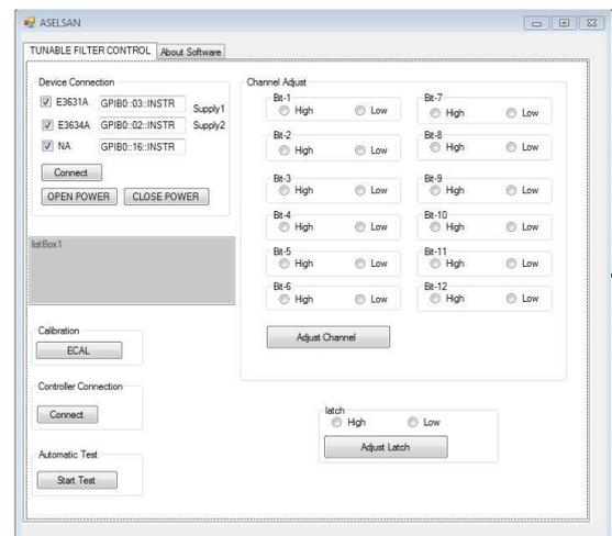
Fig.5 YIG Filter Control Interface
