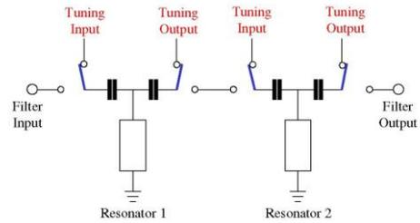
Fig.2 Resonator Based Tuning[8]
