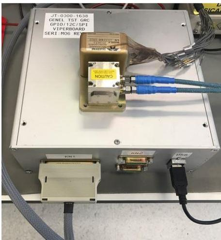
Figure 7 YIG 2-18 Notch Filter
